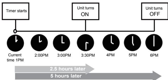
Example: If current timer is 1:00PM, to set the timer as above steps, the unit will turn on 2.5h later (3:30PM) and turn off at 6:00PM.
