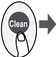
Airborne bacteria can grow in the moisture that condenses around heat exchanger in the unit. With regular use, most of this moisture is evaporated from the unit. By pressing the CLEAN button, your unit will clean itself automatically. After cleaning, the unit will turn off automatically. Pressing the CLEAN button mid-cycle will cancel the operation and turn off the unit. You can use CLEAN as often as you like.
